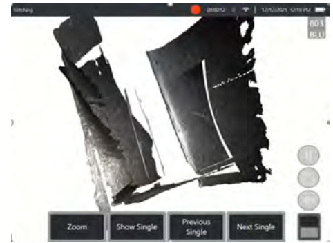
The example shows poor image registration of a compressor blade
